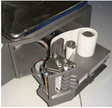
(6) Close the turnable printing assembly.
